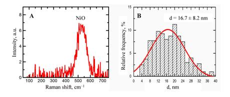
**Figure 9.** Characteristics of nickel oxide NPs produced by laser ablation. (A) Raman spectrum; (B) size distribution function obtained by statistical processing of SEM NPs images.
