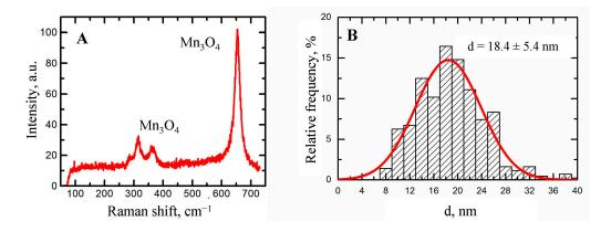
Figure 10. Characteristics of manganese oxide nanoparticles produced by laser ablation. (A) Raman spectrum; (B) size distribution function obtained by statistical processing of SEM images of NPs.
