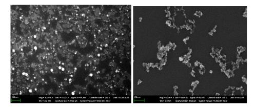
**Figure 8.** SEM images of NiO (**left**) and Mn<sub>3</sub>O<sub>4</sub> (**right**) nanoparticles in suspension obtained by scanning electron microscopy.
